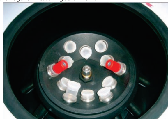
Figure 2: Centrifugation of blood using REMI R-8C laboratory centrifuge for measuring serum ferritin
